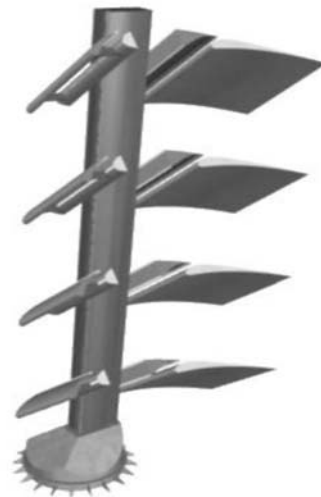
Figure 2 - High lift wing sail changing direction
