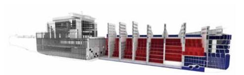
➤ basically only connected on the sides to the not-so-rigid 'torsion box' front part. This transition zone between the ship's container shape and the ro-ro shape required Finite Element (FEM) calculations that were all part of the package.
