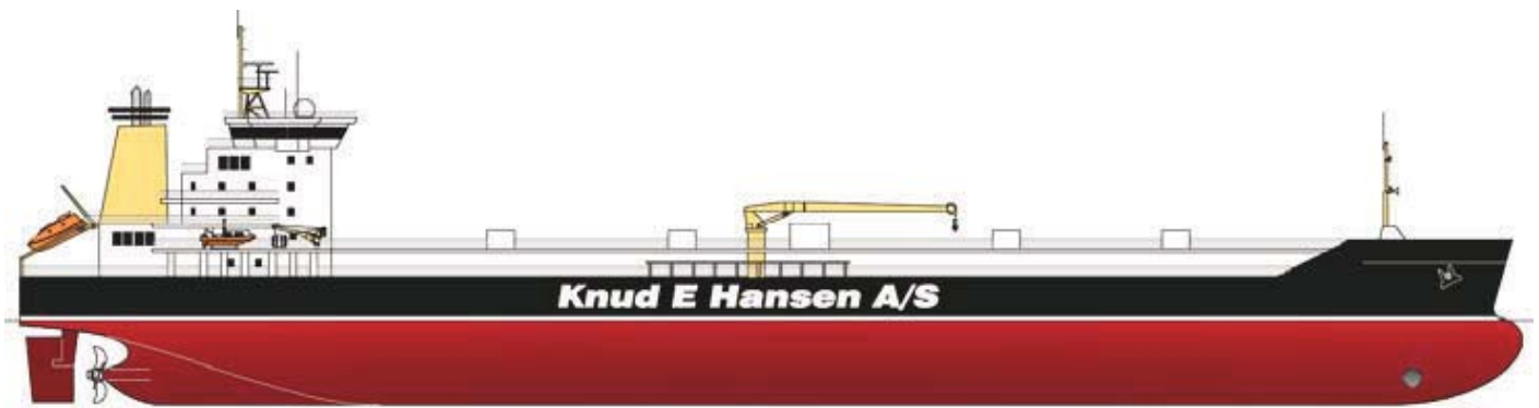
KEH's 24,000 dwt IMO II chemical tanker design.
