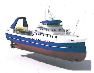
The ship is constructed to meet DNV SILENT-F requirements
