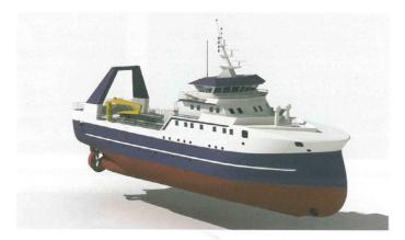
The shape of the trawler's hull form is designed to minimise both slamming and vertical accelerations.
