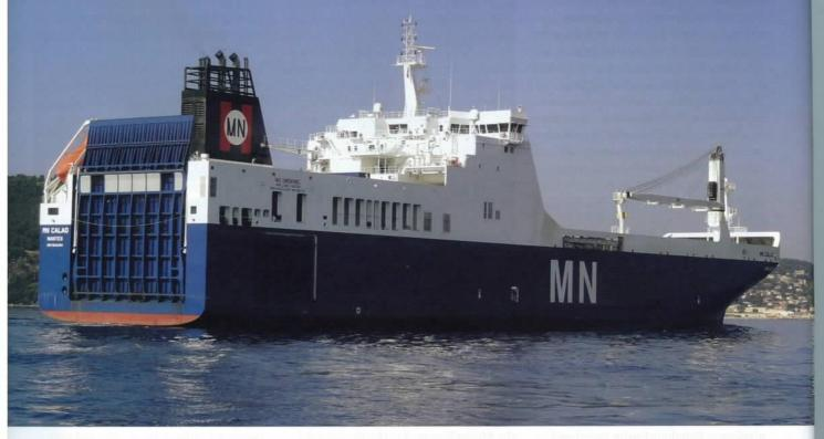
he MN CALAO is the first of two ro-ro ships delivered to the French company Maritime Nantaise (MN) by Hyundai Mipo Shipyard. Continuing the builders specialization in the construction of ro-ro vessels, the new pair are actually the smallest ro-ros that have been built by the yard but they incorporate a number of special features making them highly suitable for military logistics.
