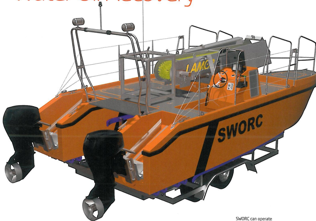
SWORC can operate in 35 cm water depth.
