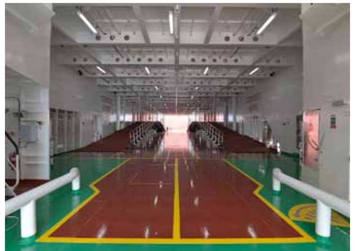
Car deck with lowered mezzanine deck.
