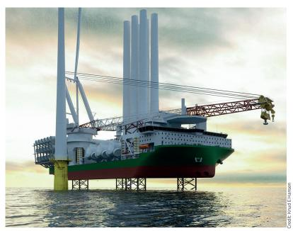
The hull elevates on four three-chorded trusswork legs, supporting the vessel, its payload and the installation process in water depths up to 80m. Raising and lowering is effected by a powerful, electrical rack-and-pinion jacking arrangement. The elevating system is designed for 5,000 load cycles, reckoned to be significantly more than many competing solutions and intended to ensure that the leg racks last the lifetime of the vessel.
