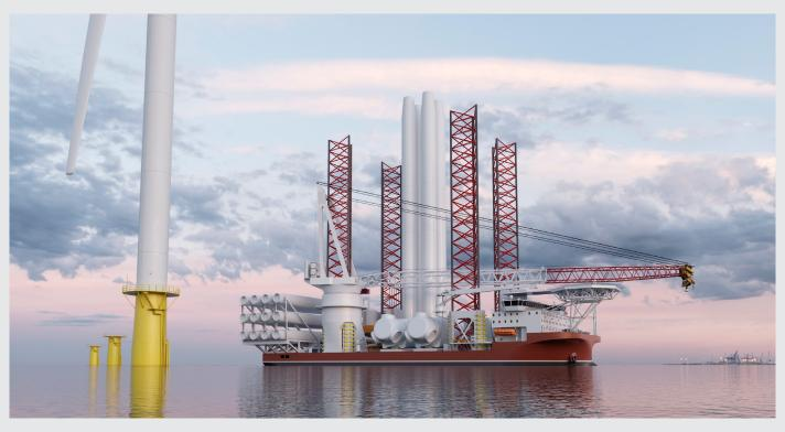
The latest addition to KNUD E. HANSEN's Atlas series of wind turbine installation vessels, the Atlas A-class is able to carry four new-generation 14 megawatt wind turbines and is tailored for cost-effective installation of large-scale wind farms.
