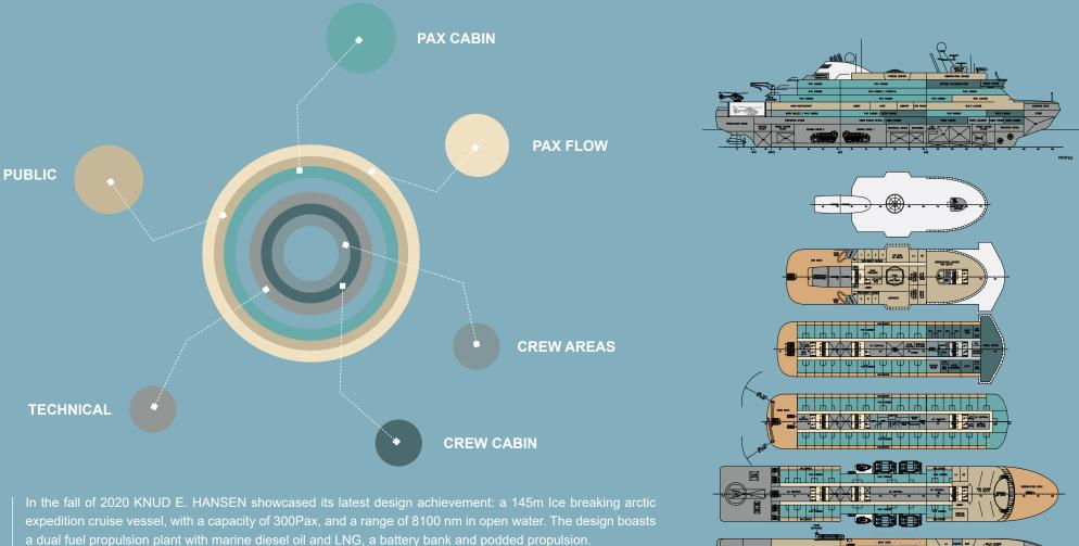
The arrangement provides superior maneuverability and efficiency with the ability to provide zero emissions while moored in some of the worlds most environmentally sensitive regions. The design has a PC3 ice class and is equipped with all necessary facilities for arctic operations.
