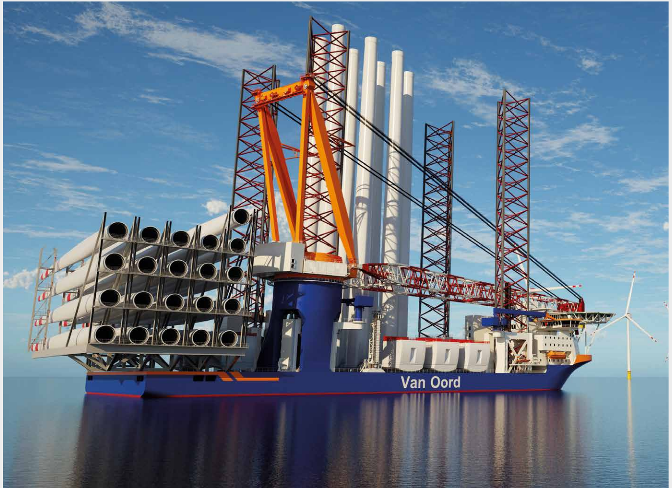
▼ 175m WTIV for Van Oord, based on the Atlas C-Class
