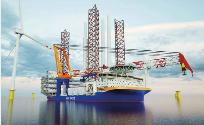
▼ 175m WTIV for Van Oord, based on the Atlas C-Class
