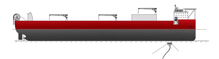
The platform is a floating storage and injection unit dedicated to liquified  $CO_2$  handling. The platform is positioned at sea and connected to injection wells via a submerged turret system.
